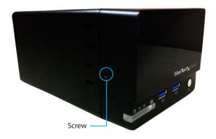
2. To reveal the drive bay, grasp the front panel and slide it upward.
